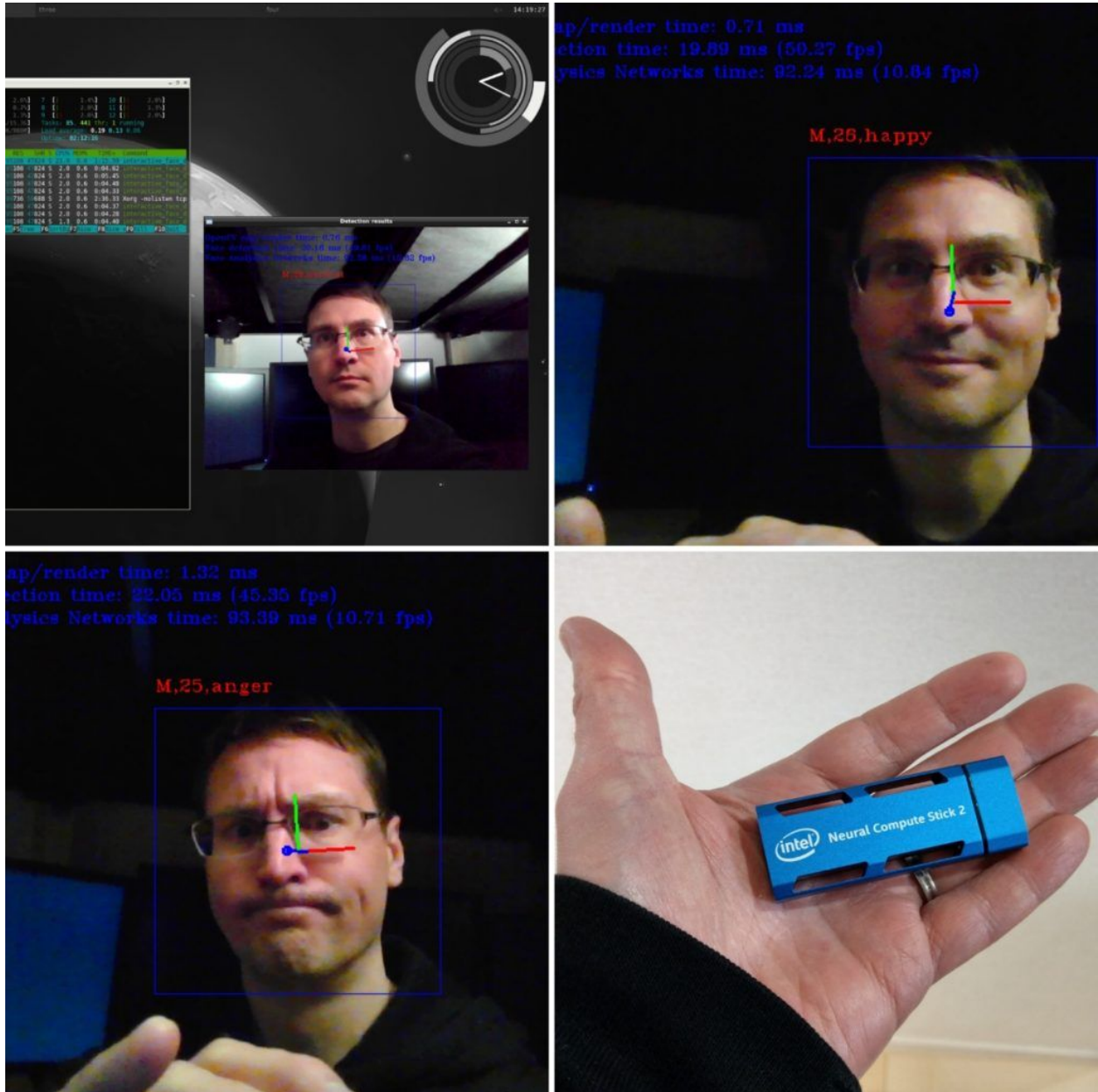
Facial, Age and Mood detection with Intel Neural Compute Stick 2
